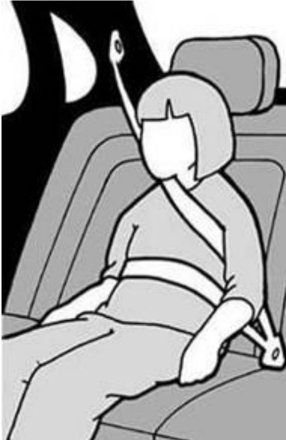
Incorrect belt fit because there is no booster seat
